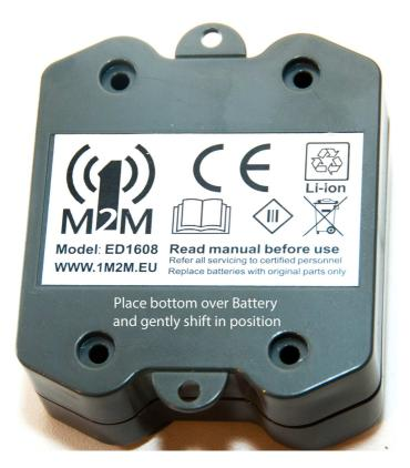
*Step 5:* Place the washers in the holes of the bottom of the enclosure and put the torx screws in the enclosures. Now you can tighten the enclosure.
